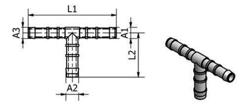
Ext. Hose Diameter A3 = 13 Ext. Hose Diameter A1 = 13 Ext. Hose Diameter A2 = 13 L1 = 69 L2 = 36
